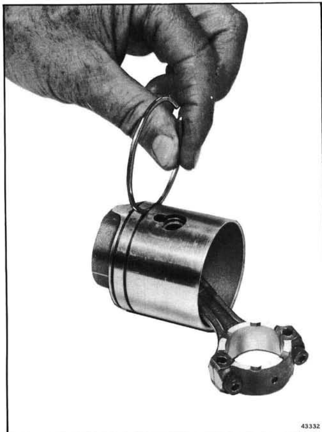
Figure 5-29. Checking Fit of Lower Ring in Groove
