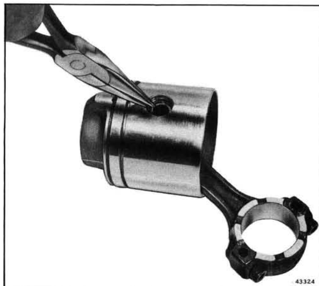
Figure 5-21. Removing Piston Pin Retaining Ring
