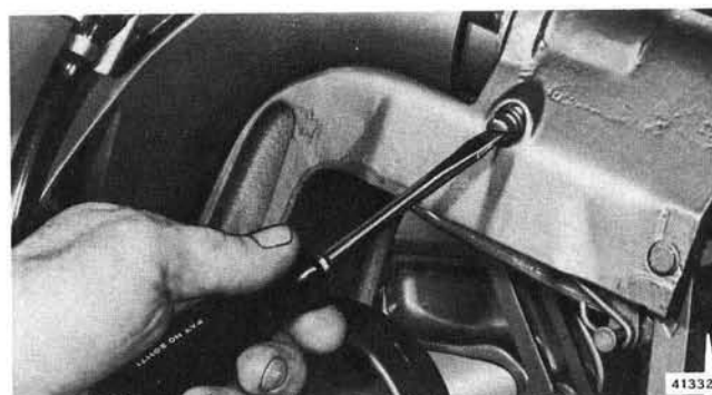
Figure 6-63. Steering Friction Adjustment
