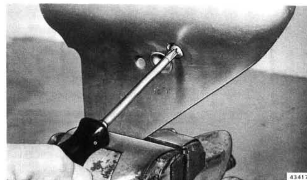
Figure 6-28. Removing Pivot Pin
