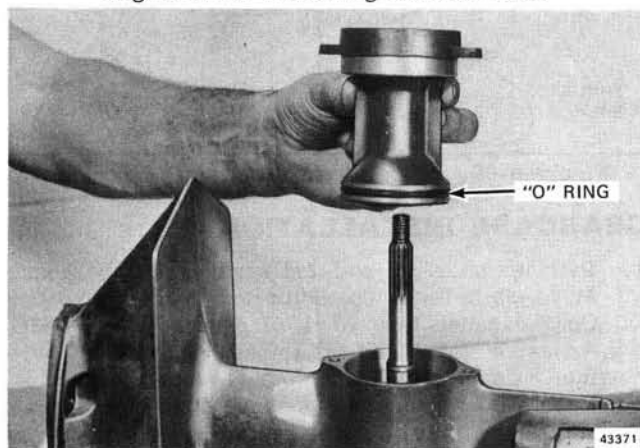
Figure 6-53. Installing Bearing Housing
