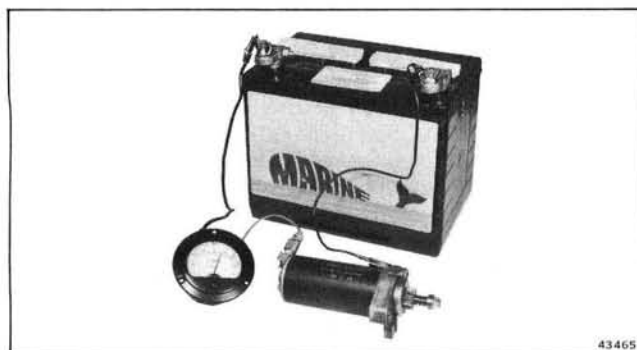
Figure 7-4. No Load Test
