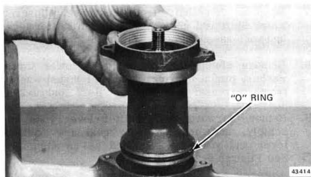
Figure 6-26. Removing Bearing Housing
